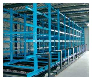
Other racking systems installed on mobile bases, e.g. Cantilever mobile
