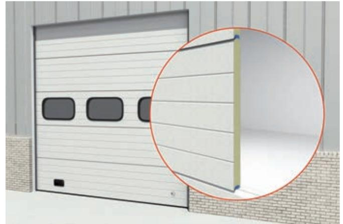
The Loading Systems traditional industrial panel is provided with an in-built thermal break. The tongue and groove design ensures an almost seamless seal between the panels preventing air and/or water from penetrating through the seals, ensuring the best possible insulation properties.
