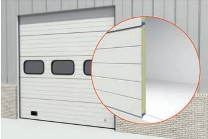
Loading Systems offers a “finger-safe” door panel profile which protects operatives from trapping their fingers between the panels when the door is operated. A finger protection device, or “finger-safe” design is legally required according to CE standards for all overhead doors with an opening height of 2750 mm or less (door panel deviates below 2750 mm).
